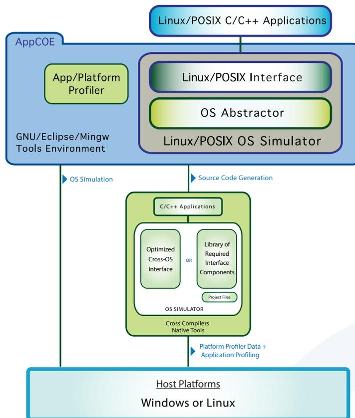
Linux/POSIX OS Simulator is integrated with AppCOE, an Eclipse-based framework packaged with CDT, BIRT and GNU x86 tools, providing a state-of-the-art IDE for development and testing. Linux/POSIX OS Simulator provides the following features when used as a development platform:
