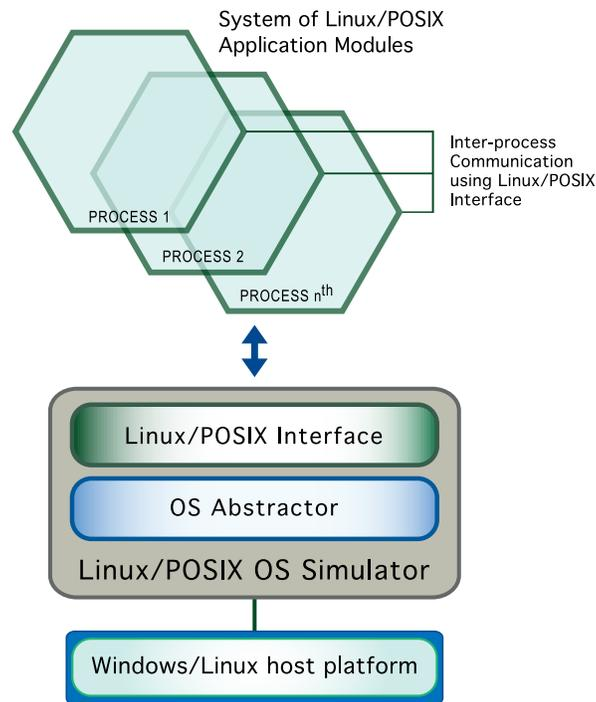
Linux/POSIX OS Simulator provides the ability to simulate, test and run an entire system of C/C++ Linux/POSIX applications on a Windows or Linux host. Host-based testing offers more hardware resources, less complexity and lower costs when compared to testing on a target platform. Linux/POSIX OS Simulator provides the following features when used as a virtualized testing platform:
